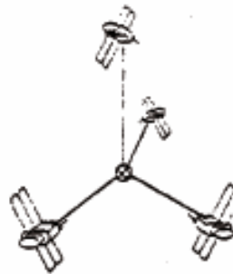
GOOD GDOP (ideal case) • one satellite overhead • 3 on horizon, 120° apart in azimuth
